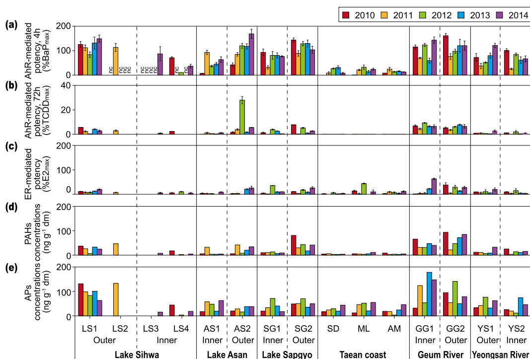
Fig. 2. AhR-mediated potencies after (a) a 4-h exposure and (b) a 72-h exposure using the H4IIE- luc bioassay; (c) ER-mediated potency using the MVLN assay, and distributions of (d) PAHs and (e) APs in sediments along the west coast of South Korea from 2010 to 2014.
